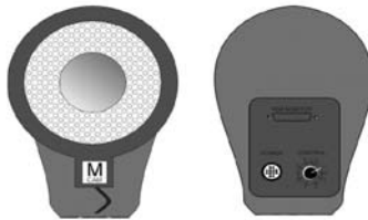
Figure 2.1: The MCam2 style of camera. Front and rear panel. Image Courtesy of VICON Motion Systems, OMG Plc. Source Tebbutt, Wood and King (2002).
